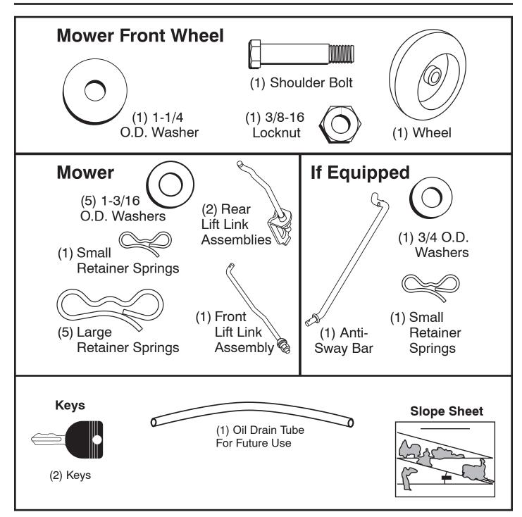
Your new tractor has been assembled at the factory with exception of those parts left unassembled for shipping purposes. To ensure safe and proper operation of your tractor all parts and hardware you assemble must be tightened securely. Use the correct tools as necessary to ensure proper tightness.
